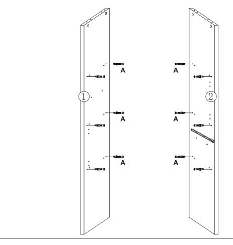
STEP 7: Attach panels (1)(2) to the body with dowel(C) and cam lock parts.
